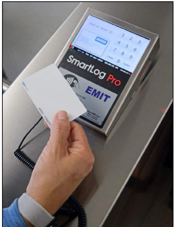
Figure 5. Holding a proximity badge in front of the RFID icon on the SmartLog Pro™
