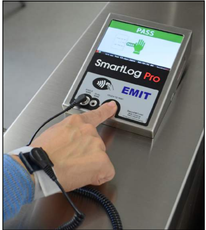
Figure 7. Performing a single-wire wrist strap test
