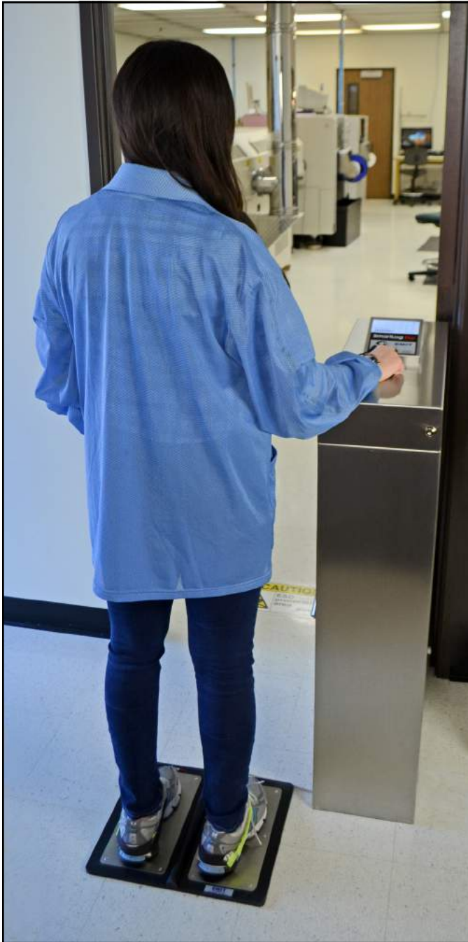
Figure 6. Performing a footwear test
