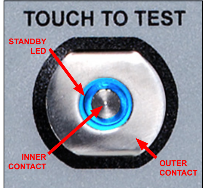
Figure 3. Steady-State Test Switch features and components
