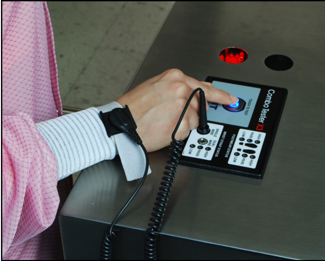
Figure 4. Bridging the test switch's contacts to initiate the test
