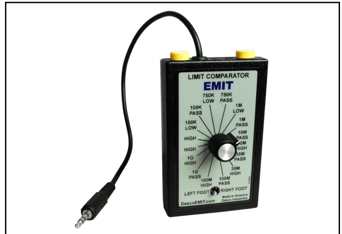
Figure 5. EMIT 50424 Limit Comparator
